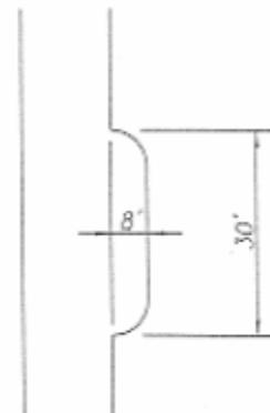
Figure 4. Parking bays should be provided where on street parking is needed and the requirements for additional grading are minimal.
