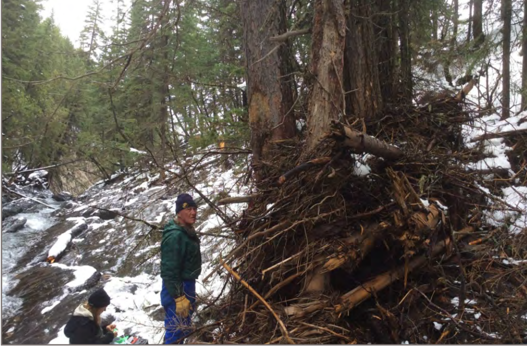
Photo 213(2): Log jam against trees and flood damage on trees above jam. The logs and damage are from the 2013 event and show the minimum flood level above the current creek surface. Looking north with waterfall drop off in background.
