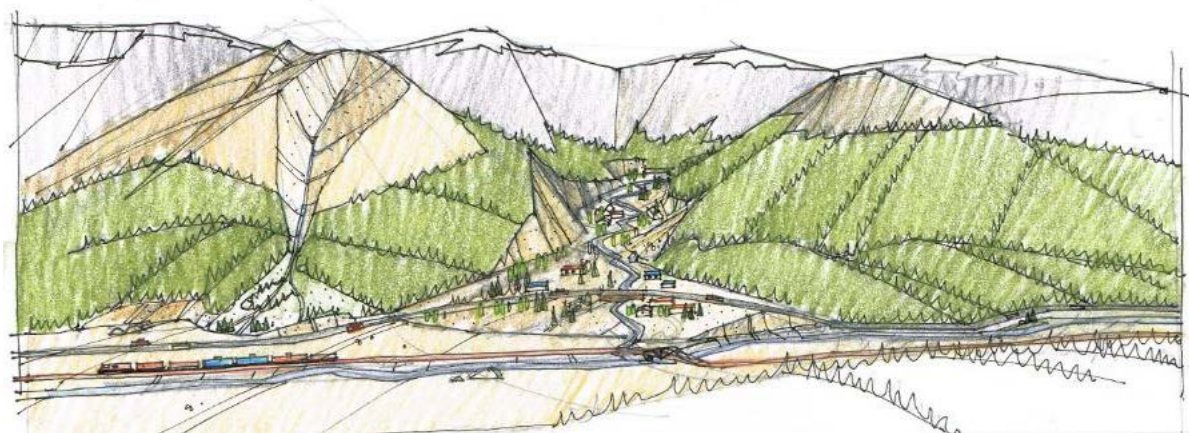
Figure A-2. Typical steep and low-gradient fans feeding into a broader floodplain. On the left a small watershed prone to debris flows has created a steep fan that may also be subject to rock fall processes. On the right a larger watershed prone to debris floods has created a lower gradient fan. Development and infrastructure are shown to illustrate their interaction with steep creek geohazard events. Artwork: Derrill Shuttleworth.
