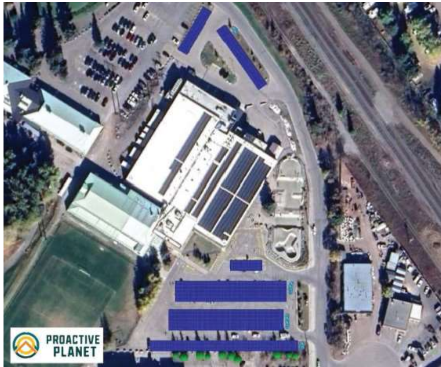
Figure 4.5: Preliminary Module Layout - Canmore Recreation Centre Parking Lot
