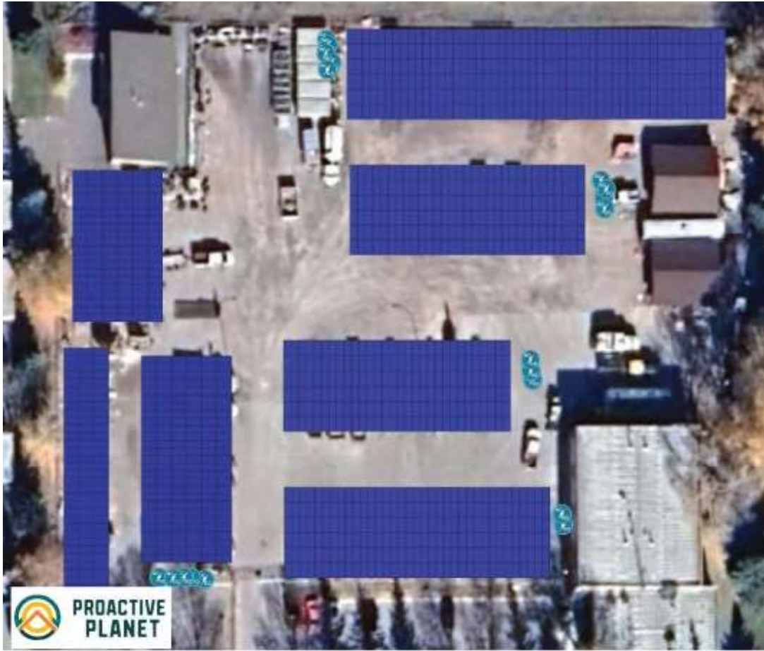
Figure 4.13: Preliminary Module Layout - Public Works Yard
