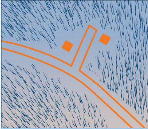
Inappropriate dead-end access
