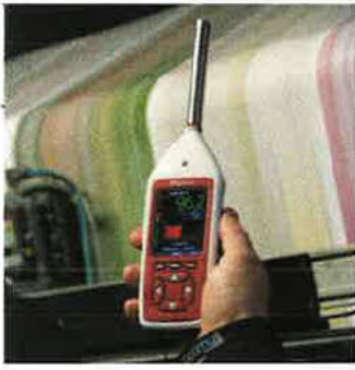
Example of a Type 1 sound level meter.
