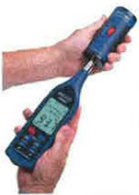
Image showing calibration process.
