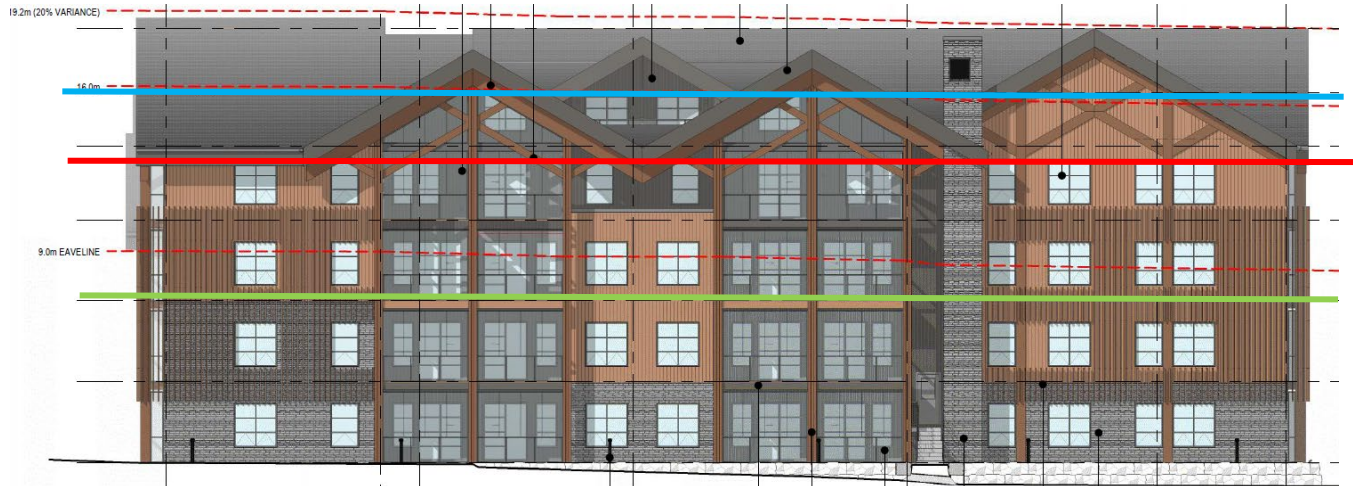
Figure 3: Side (West) Elevation Showing 7.0m Maximum Eaveline Height in Green, Proposed 13.0m Eaveline Height in Red and 16.0m Maximum Building Height in Blue
