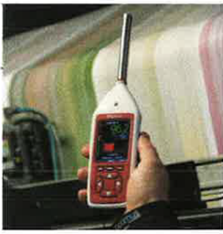
Example of a Type 1 sound level meter.
